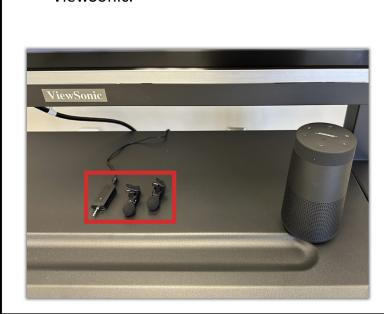
Press and hold the power button on both the microphone and the audio receiver. An indicator light will illuminate on both devices. When the microphone has paired with the receiver the microphone will have a green light present and a blue light will be present on the receiver. (Battery life approx. 5 hours)
